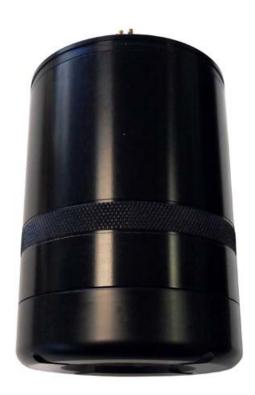
The Imagenex Model 862 is a completely self-contained altimeter with analog output. It is mounted in a pressure proof housing with an underwater connector for use at depth. The 862 Altimeter measures the range to the bottom or other large objects. It requires only power and an analog interface to an external device.
